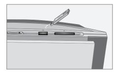
1 Connect the USB interface of the MP3 player to the »USB« socket of the device with a standard USB cable;
